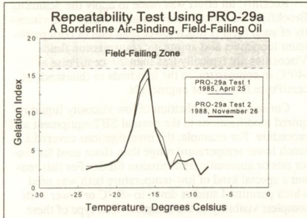
Fig. 10 - Gelation Index curves for a borderline, field-failing oil run twice by different operators on different instruments three and one-half years apart.
