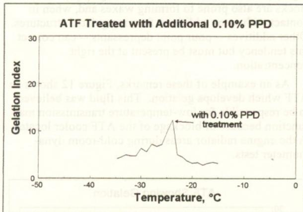
Fig. 14 - Comparison of the effect of doubling amount of added PPD in the treated ATF Gelation Index curves remain essentially the same as for the ATF of Figure 12.
