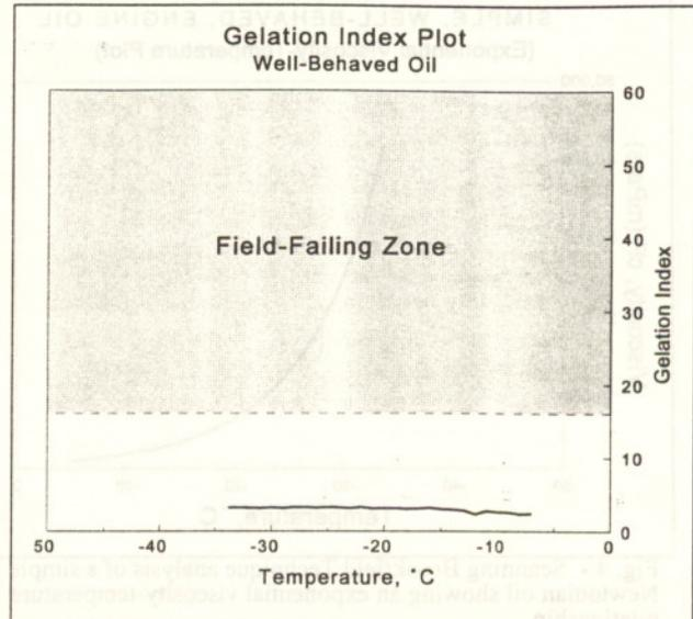
Fig. 8 - First derivative of the MacCoull, Walther, Wright plot for the well-behaved engine oil shown in Figure 6.
