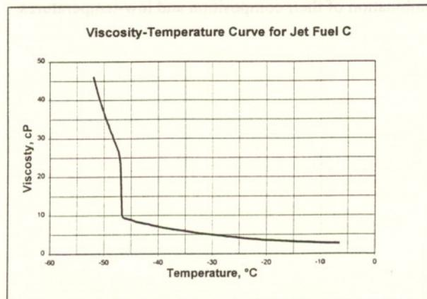
Fig. 20 - Viscosity-temperature curve of Jet Fuel C
