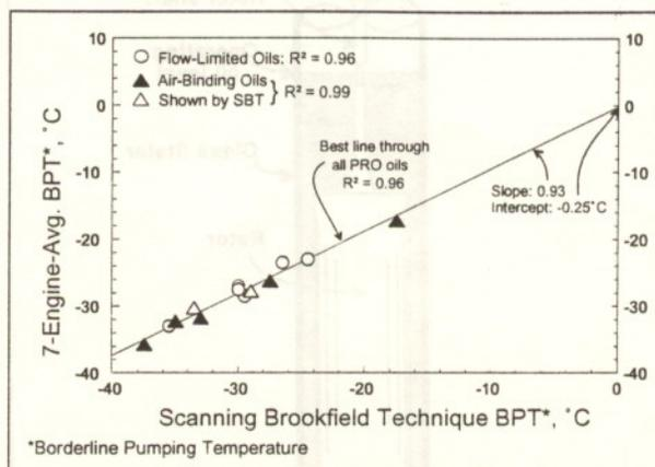
Fig. 1 - Correlation of SBT-determined borderline pumping temperatures with those obtained in cold-room engine
