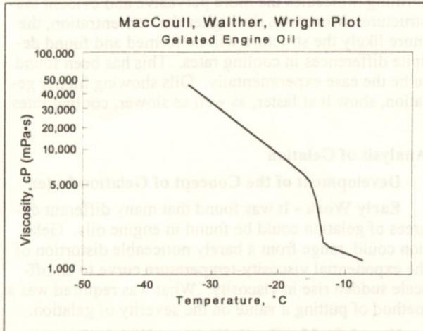
Fig. 7 - MacCoull, Walther, Wright plot of the viscosity-temperature data of a mildly gelled engine oil.
