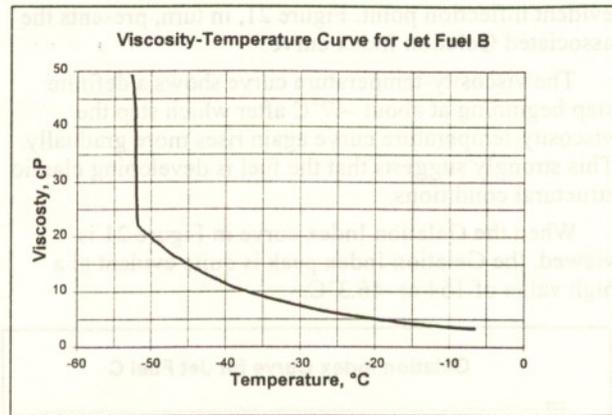
Fig. 18 - Viscosity-temperature curve of Jet Fuel B
