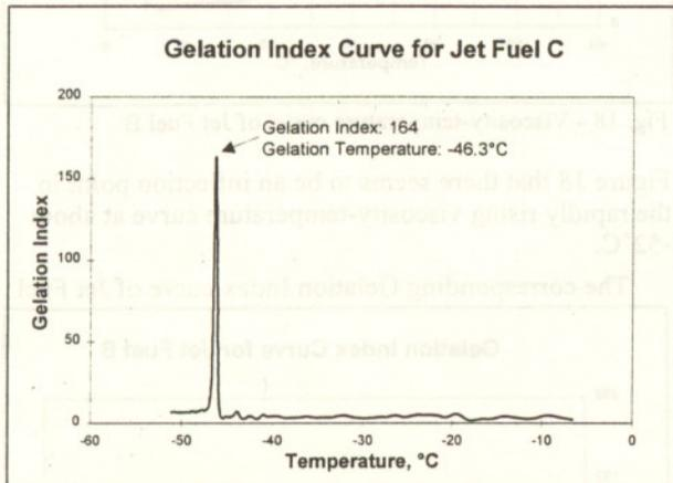
Fig. 19 - Gelation Index curve of Jet Fuel C showing evident gelation effects at  $-46.3^{\circ}\text{C}$ .
