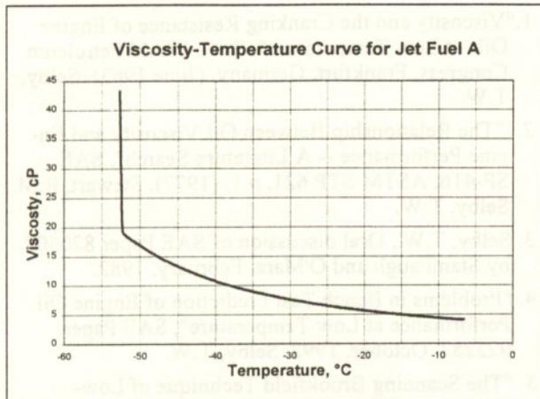
Fig. 16 - Viscosity-temperature curve of Jet Fuel A
