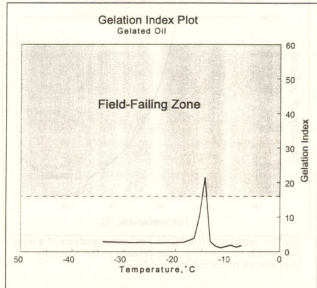
Fig. 9 - First derivative of the MacCoull, Walther, Wright plot for the gelled engine oil shown in Figure 7.
