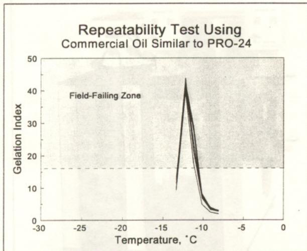
Fig. 11 - Gelation Index curves for a field-failing oil run simultaneously in seven different test cells by the same operator show good repeatability.
