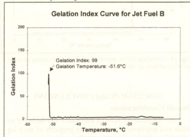
Fig. 19 - Gelation Index curve of Jet Fuel B. Also shown is the sharp Gelation Index of 99.
