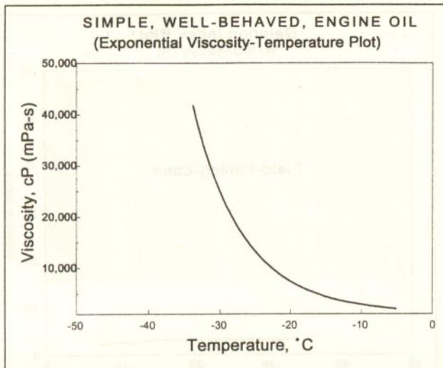
Fig. 4 - Scanning Brookfield Technique analysis of a simple Newtonian oil showing an exponential viscosity-temperature relationship
