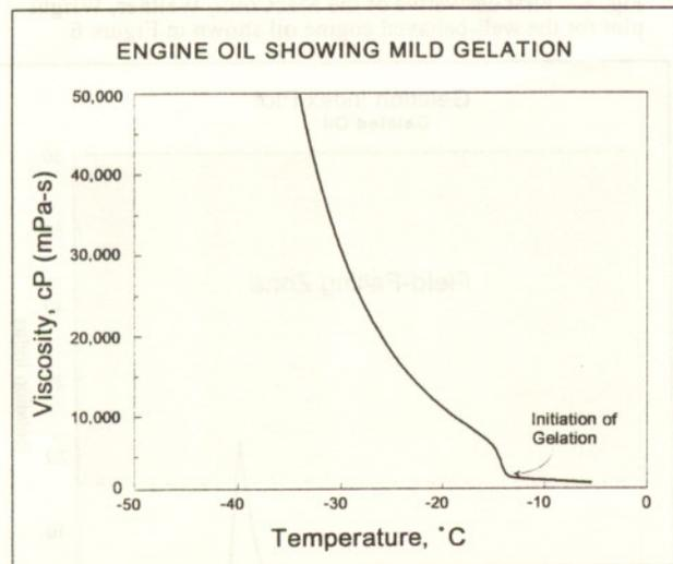
Fig. 5 - Scanning Brookfield Technique analysis of a non-Newtonian oil showing some gelation in the viscosity-temperature relationship at  $\sim -12^{\circ}\text{C}$ .
