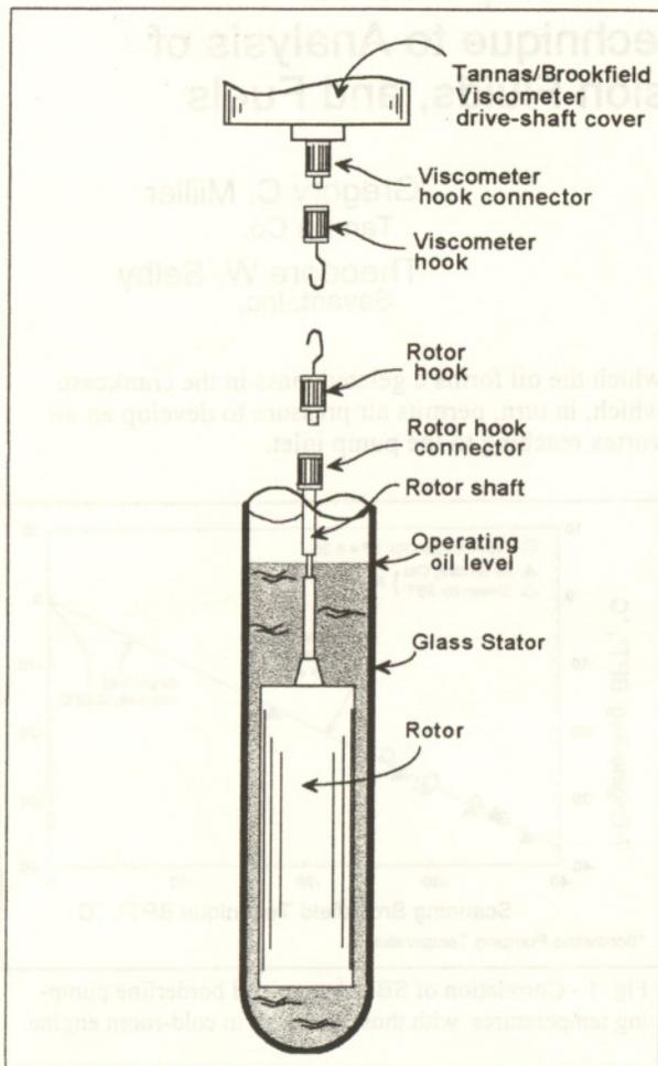
Fig. 2 - Sketch of Scanning Brookfield Viscometer rotor/stator assemblage.
