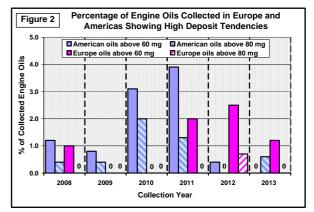
the evident improvement shown in 2012 and 2013 for the oils marketed in the Americas. With some level of contrast, in Europe where the turbocharger bench test is not a required specification for the engine oils produced, the marketed oils sampled show some increase in the presence of deposit-susceptible oils for 2012 and 2013.
