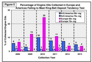
The data shown in Fig. 5 give both concern and hope – concern up to 2010 regarding both the Americas and Europe (particularly the latter) – and hope from 2010 on as the level of serious failure drops rapidly. Forthcoming IOM collections from both areas should be very interesting to evaluate and compare.
