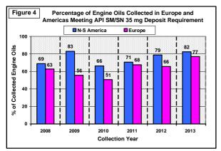
Fig. 4 shows the percentage of the oils collected each year from both Europe and the Americas that meet the criteria of a maximum of 35 mg. Since the ILSAC/API specification of SN in late 2010 both Europe and the Americas have shown increase in the number of engine oils meeting the 35 mg maximum deposit level for the TEOST MHT ring-belt deposit test. Europe improved from 51% to 77% and the Americas from 66% to 82%.
