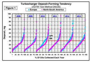
It should be noted that near the end of 2010 the American Petroleum Institute issued the latest Standard SN for the engine oils. The new standard was an upgrade of the previous Standard SM and included the requirement to have a deposit level of 30 mg or less in the ASTM D6335 test for turbocharger deposit tendency. This new requirement is also shown in Fig. 1 as a horizontal red line.
