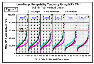
The SAE J-300 Engine Oil Viscosity Classification requirement of a viscosity level no greater than 60,000 mPa•s (cP) is also shown. Using this criterion of acceptability, the Americas show considerably better response to the test with the exception of 2013. It is likely that this pattern reflects the long North American concern with pumpability since Sioux Falls and the recent adverse European experience of 2008-2009.
