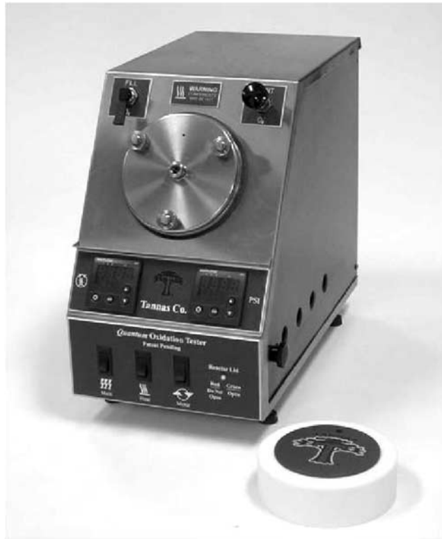
FIG. 2—Bench top, dry-bath RPVOT and lid cover.
