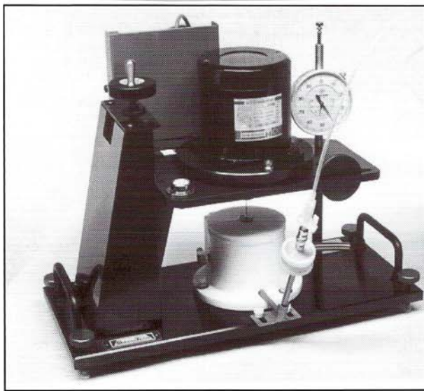
Figure 5 - Model 400 Tapered Bearing Simulator-Viscometer for very high shear rate rotational viscometry.
