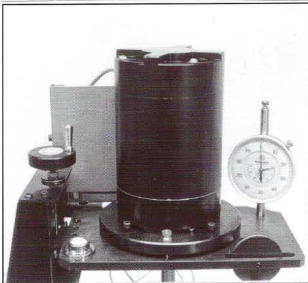
Figure 6 - Motor of Model 600 Tapered Bearing Simulator-Viscometer for high shear rate viscometry above 12 cP.
